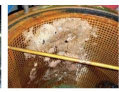
Normex validated the performance in preventing settlement of marine organisms on the inlets to the sea chest and the heat exchanger at different ozone doses. During the validation they also monitored the formation of bromates.
