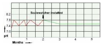
A graphic illustration of the actual reduction in Chlorine, whilst the graph shows the stability of pH, without the addition of chemicals, following the installation of the Scalewatcher at a municipal pool.
