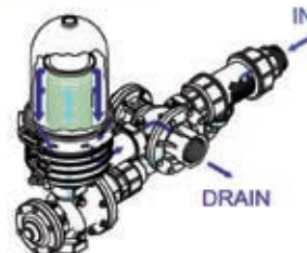
Filter in Backwash mode
